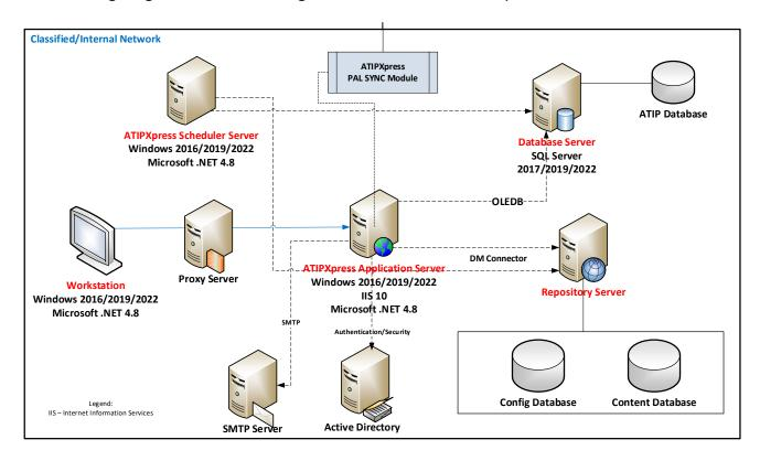
(!!) Note: The ATIPXpress application and all other components can be installed on a single server if the organization size and workload are minimal. However, it is highly recommended to house the database, application and scheduler on separate servers due to the high volume of processing required by the CPU.
